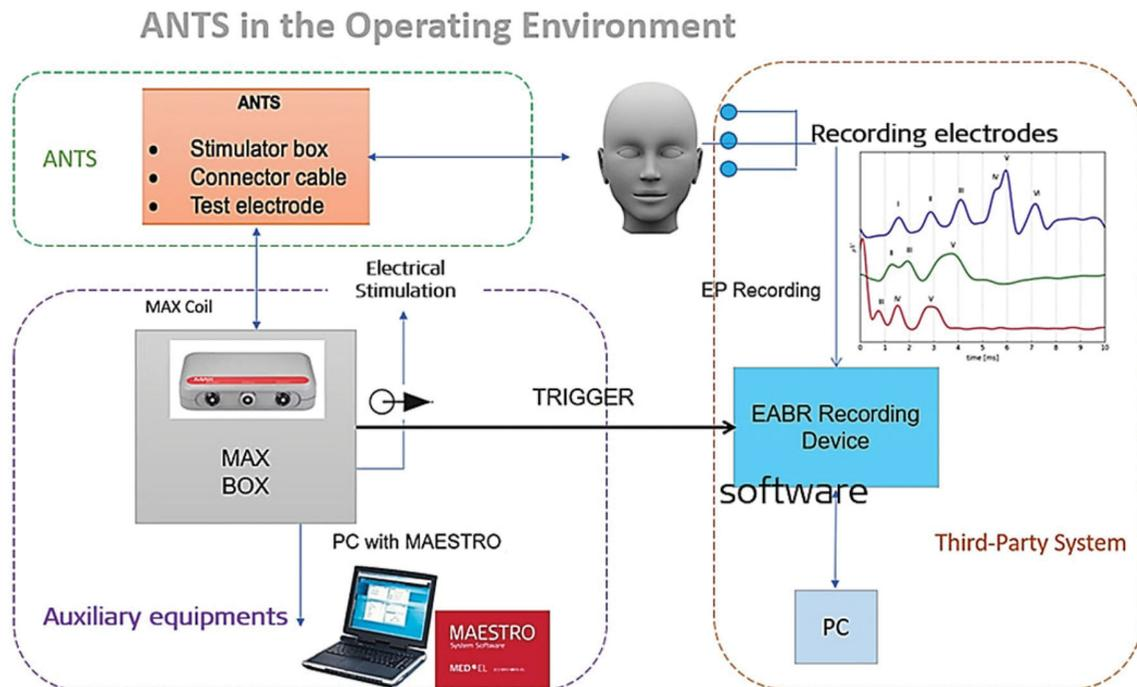
Figure 27. Intracochlear test electrode and test set-up in recording the eABR responses (image courtesy of MED-EL).
