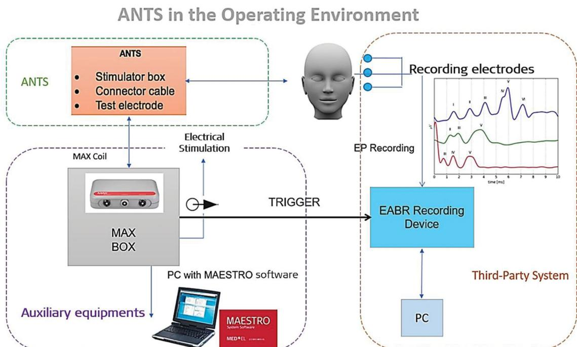
**Figure 24.** Test set-up in applying the test electrode and in recording the eABR responses. Image courtesy of MED-EL.
