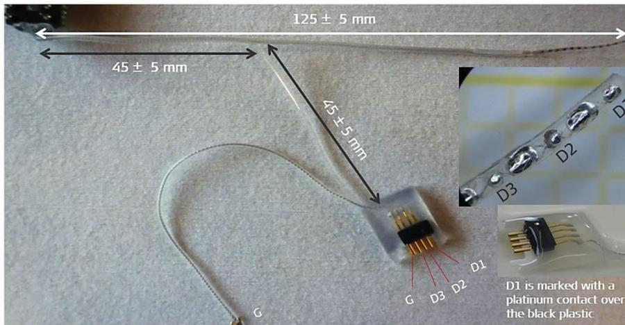
**Figure 38.** Electrode array that carries three additional diagnostic channels at the apical end of the electrode array. The diagnostic contacts are wired separately and have its connector for connecting it to external devices to record the cochlear microphonics. Image courtesy of MED-EL.
