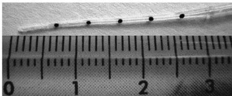
**Figure 31.** Silicone dummy of a STANDARD electrode array from MED-EL, with an open channel that runs through the length of the array (image courtesy of MED-EL).
