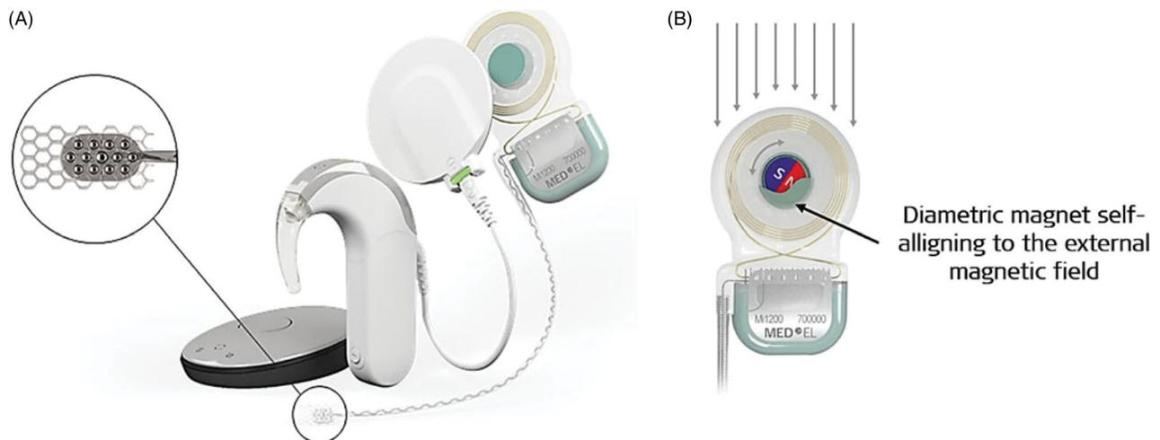
Figure 18. SYNCHRONY ABI system showing both single unit and BTE audio processor (A). The implant has a 1.5T conditional MRI compatible magnet that self-aligns to the external magnetic field (B) (image courtesy of MED-EL).
