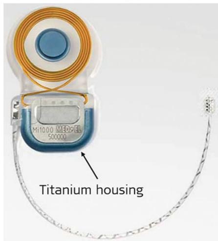
**Figure 12.** CONCERTO ABI implant system with titanium housing encasing the implant electronics (image courtesy of MED-EL).
