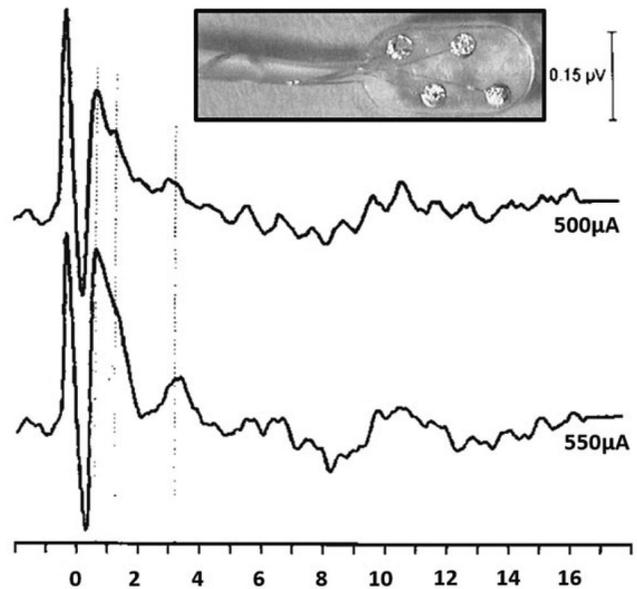
**Figure 7.** MED-EL's ABI placement/test electrode with four stimulating contacts and waves in eABR recording (image courtesy of Prof. Behr) [5].
