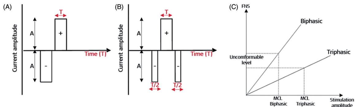
**Figure 52.** Balanced biphasic pulse stimulation (A) and triphasic pulse stimulation (B) showing two negative phases of duration ( $T/2$ ) and one positive phase duration ( $T$ ) (image courtesy of MED-EL). Model of expected benefit with triphasic pulse stimulation on FNS (C) (image recreated from Bahmer et al. [44]).
