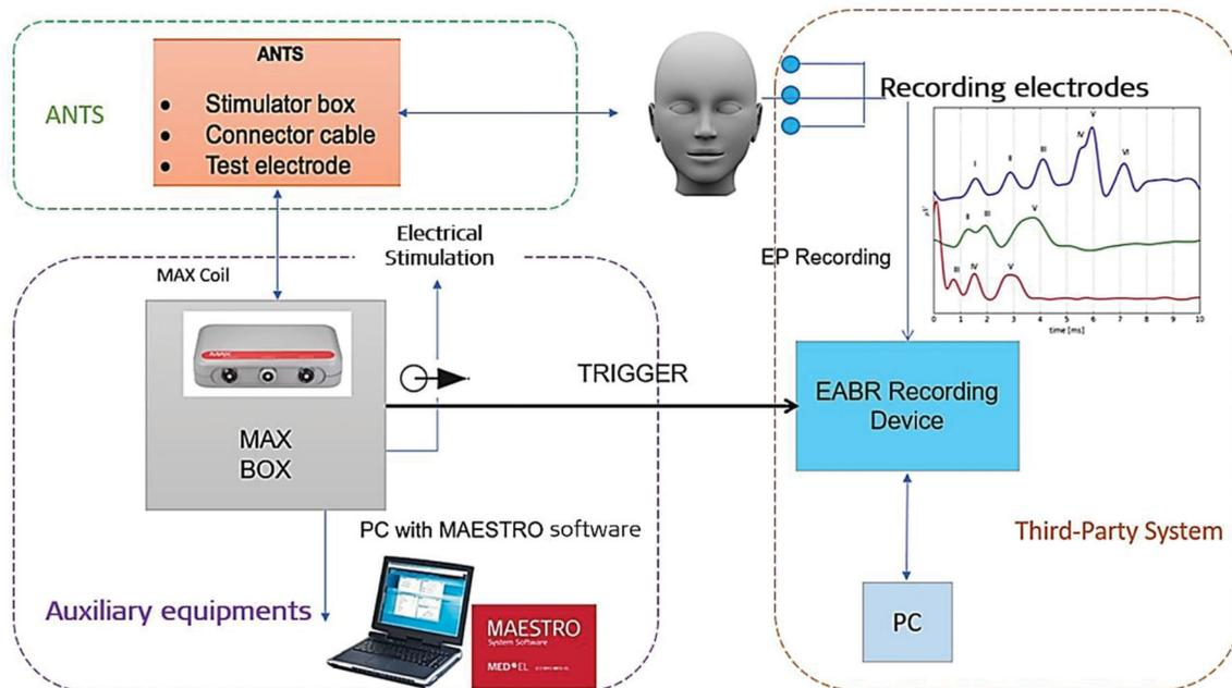
Figure 24. Test set-up in applying the test electrode and in recording the eABR responses. Image courtesy of MED-EL.
