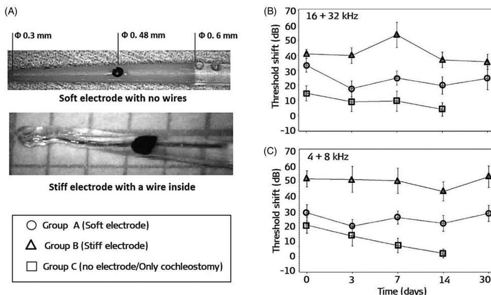
**Figure 8.** Soft and stiff electrodes fabricated by MED-EL for this study (A). Average threshold shifts in dB SPL at the high-frequency band (16 + 32 kHz) (B) and at low-frequency bands (4 + 8 kHz), (C) measured immediately after the surgery ( $t = 0$  days) and at  $t = 3, 7, 14$  and 30 days postoperatively [16]. Statistical analysis: unpaired  $t$ -test ( $p < .05$ ). Reproduced by permission of Wolters Kluwer Health, Inc.
