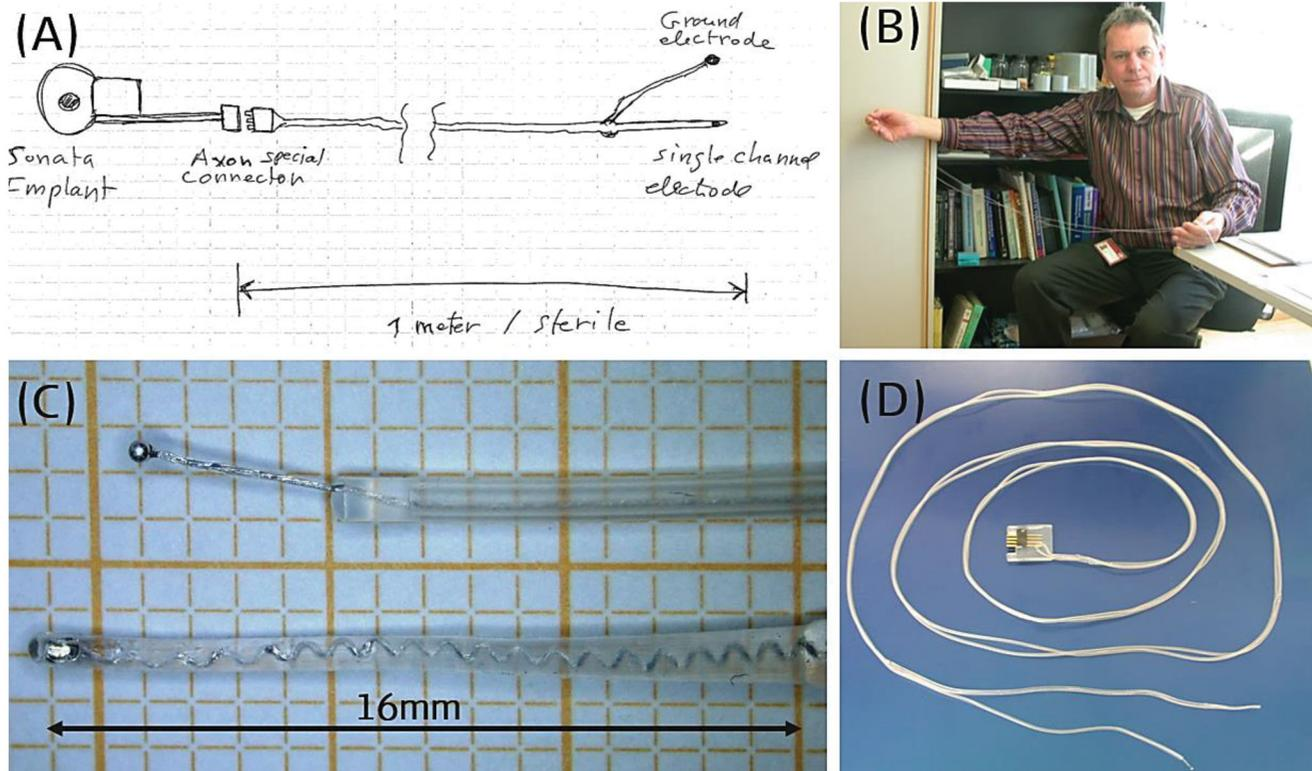
**Figure 21.** The concept of intracochlear test electrode from paper (A) to prototype (C, D), Dr. Jolly (MED-EL) holding the prototype (B). Image courtesy of MED-EL.
