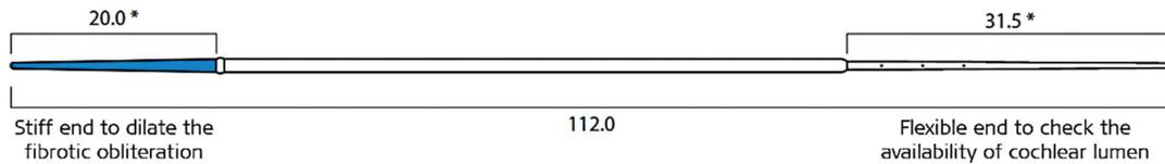
**Figure 36.** Insertion probe device with two different ends. The short blue coloured end is made stiff for a length of 20 mm to dilate the fibrous obstruction, whereas the long end is made as flexible as MED-EL's FLEX electrode arrays to check the depth of the cochlear lumen. \* Dimensions in millimetre. Image courtesy of MED-EL.
