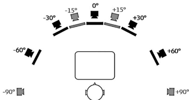
**Figure 25.** Sound localisation test setup with a child seated in front of the table and facing the centre of the arc of loudspeakers. Active (black) and inactive (grey) loudspeaker positions are shown in degrees azimuth; negative angles denote locations to the left, and positive angles denote locations to the right of the centre [36]—statistical analysis: Linear multivariable regression model.
