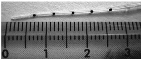
**Figure 31.** Silicone dummy of a STANDARD electrode array from MED-EL, with an open channel that runs through the length of the array (image courtesy of MED-EL).
