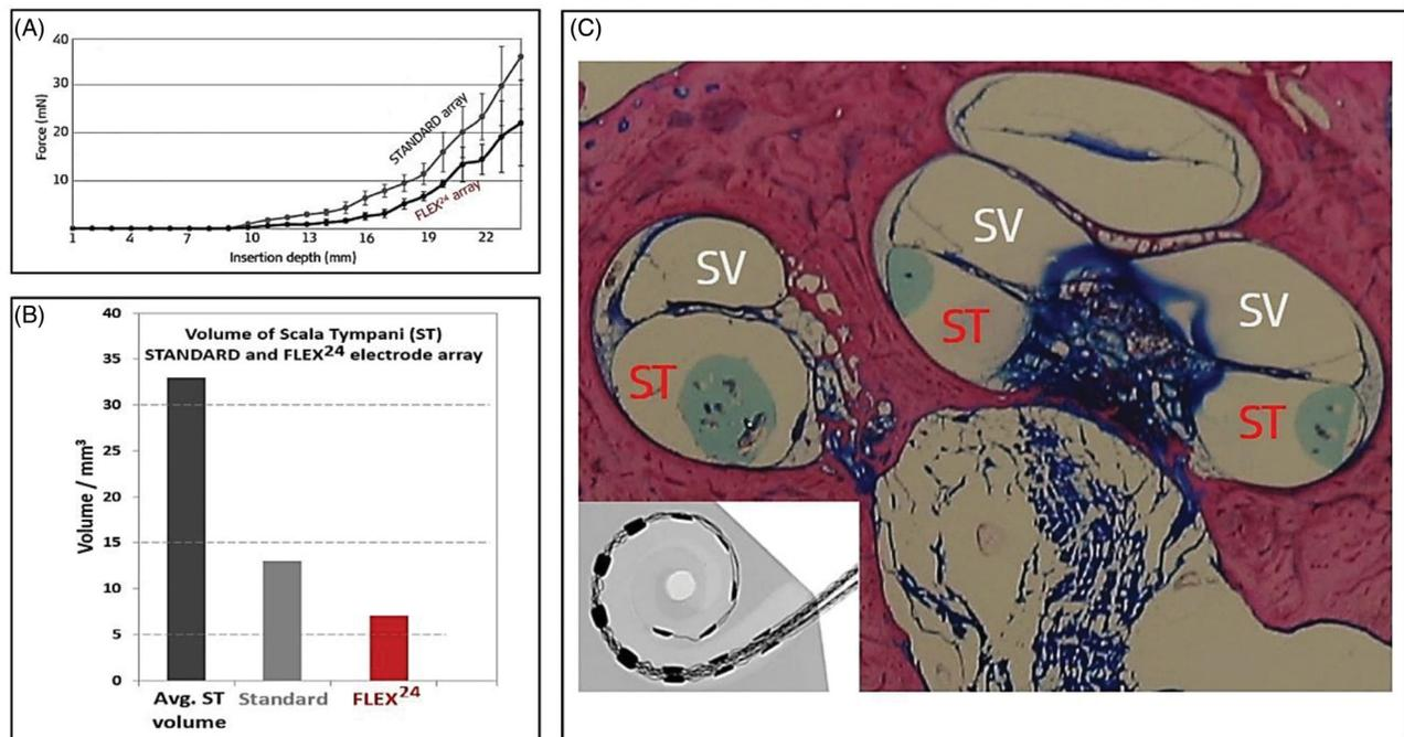
**Figure 12.** Force measurement data is showing 40% lower values for FLEX24™ electrode array in comparison with the STANDARD electrode array (A) (Courtesy of MED-EL). Mean ST volume compared against STANDARD and FLEX24™ electrode arrays—a later finding from the year 2020 (B) [11]. Histological evaluation of FLEX24™ in human cochlea, showing complete ST placement (C) [9]. Histological image—Courtesy of Freiburg Medical University, Germany, Study sponsored by MED-EL.
