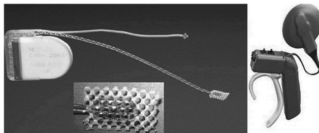
**Figure 5.** MED-EL's C40+ ABI system with paddle electrode and externally worn TEMPO + BTE speech processor (image courtesy of MED-EL).
