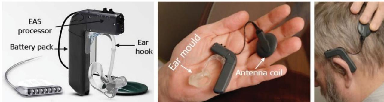
**Figure 14.** DUET™ unified audio processor (image courtesy of MED-EL).
