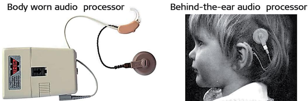
**Figure 3.** MED-EL's body-worn audio processor before 1991 and the world's first BTE audio processor in 1991 (image courtesy of MED-EL).
