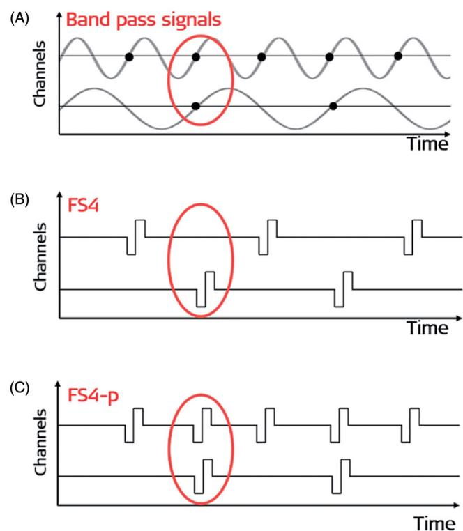
**Figure 23.** Zero-crossing of the bandpass output (A). FS4 strategy with single-pulse CSSS. In the event of zero-crossings coinciding on two or more FS channels, FS4 picks the channel with the highest instantaneous pulse amplitude for stimulation (B). The FS4-p strategy provides simultaneous stimulation pulses on two channels with coinciding zero crossings (C). Image courtesy of MED-EL.
