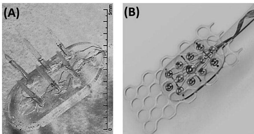
**Figure 3.** ABI paddle electrode with penetrating needle contacts (A) and flat contacts (B) (image courtesy of MED-EL).
