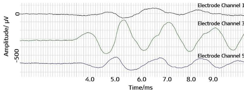
Figure 54. Prof. Artur Lorens led the study in measuring CM directly from the CI during CI surgery. Example of intracochlear ECoChG recordings for tone pips and clicks from electrode channels 1, 3, and 5 [56].
