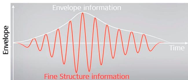
Figure 9. Simple illustration of the envelope and fine structure components of a sound signal (image courtesy of MED-EL).
