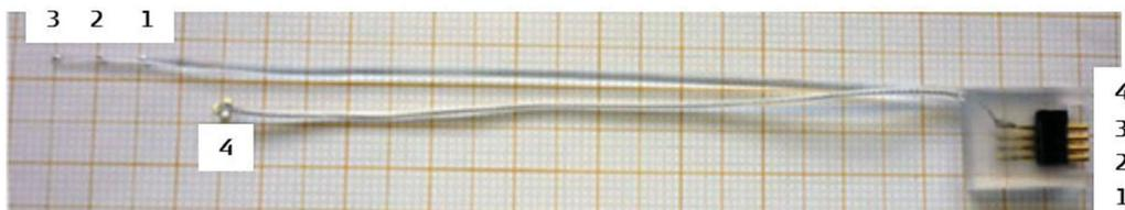
**Figure 22.** Final version of human intracochlear test electrode. Image courtesy of MED-EL.
