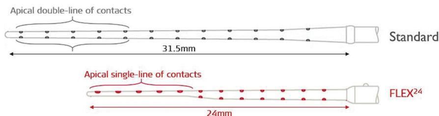
**Figure 8.** Illustration of STANDARD electrode array with apical double-lined channels and FLEX24™ electrode array with apical single-lined channels (image courtesy of MED-EL).
