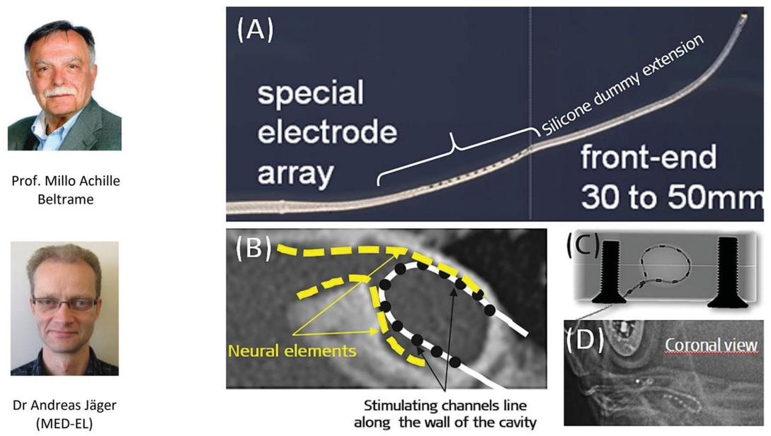
**Figure 11.** Special electrode array with silicone dummy extension conceptualised by Prof. Beltrame and realised by Dr. Andreas Jäger (A). Neural elements are believed to be present along the cavity wall, as shown by the yellow dotted line (B). X-ray image of the special electrode in a plastic cavity model (C); postoperative image showing special electrode inside the CC type cochlea (D). Image (D) courtesy of Dr. Mary Shanks, Kilmarnock.
