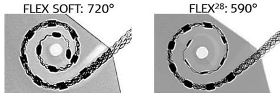
Figure 43. Angular insertion depth of FLEXSOFT™ and FLEX28™ electrode arrays in an average-sized cochlear model (image courtesy of MED-EL).
