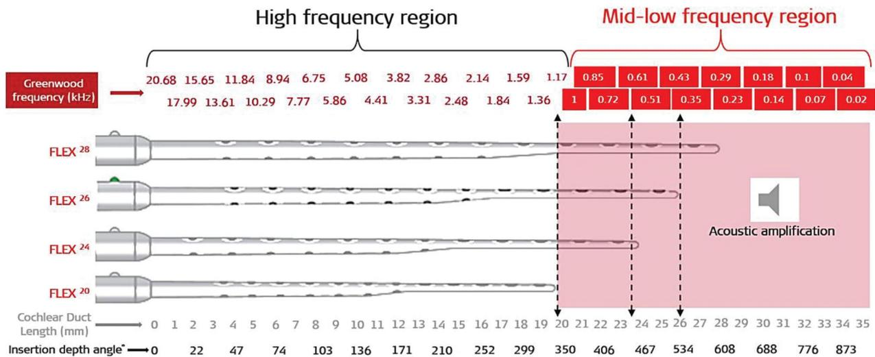
**Figure 47.** Illustration of Greenwood's frequency map for an average CDL of 35 mm with an assumption of low frequency functional residual hearing, starting at 1,000Hz. Visualisation of different electrode array lengths shows how many channels would be in the acoustic amplification zone (image courtesy of MED-EL).
