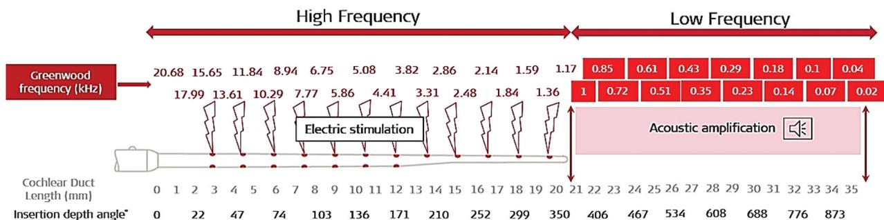
**Figure 2.** Schematic representation of electric stimulation in the HF region and acoustic amplification in the LF region in an average-sized cochlea (image courtesy of MED-EL).
