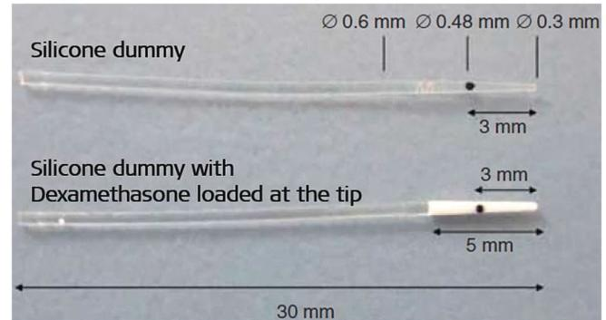
**Figure 16.** Silicone-made CI electrode dummies for non-human subject implantation with and without DEX load. The black dot indicates the insertion depth of 3 mm (Image courtesy of MED-EL).
