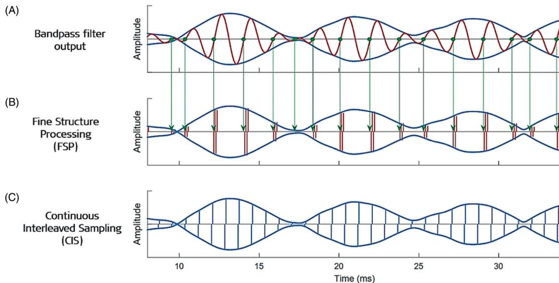
Figure 11. Differences between CIS and fine structure stimulation. Band-pass filter represents the original filtered signal, and the blue line represents the envelope function (A). Fine structure stimulation applies pulses at zero crossings of the band-pass output with an amplitude according to the envelope function (B). CIS stimulates at a fixed stimulation rate according to the envelope function (C). Image courtesy of MED-EL.
