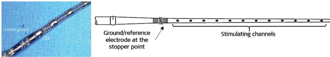
Figure 39. Electrode array that carries a reference electrode at the stopper point. Image courtesy of MED-EL.
